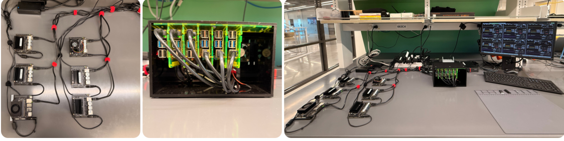
Figure 3: Real devices’ setup: 3 Raspberry Pi 4, 3 Raspberry Pi 5, 5 Jetson Nano, and 1 Jetson Orin-Nano.
